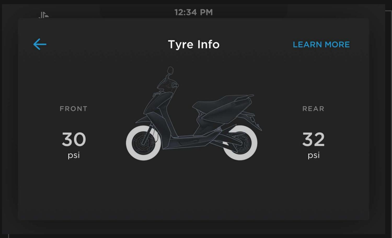
A warning symbol
